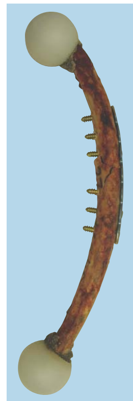
Figure 1: Overview of cadaveric bone testing model.
